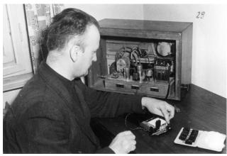
Photograph taken by the former GDR MfS of a 'Camera' transmitter as it might have been used by an agent. Note a box with spare crystals for operation on alternative frequencies.
